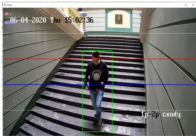
Fig. 10. An example of human recognition and tracking down the stairs
