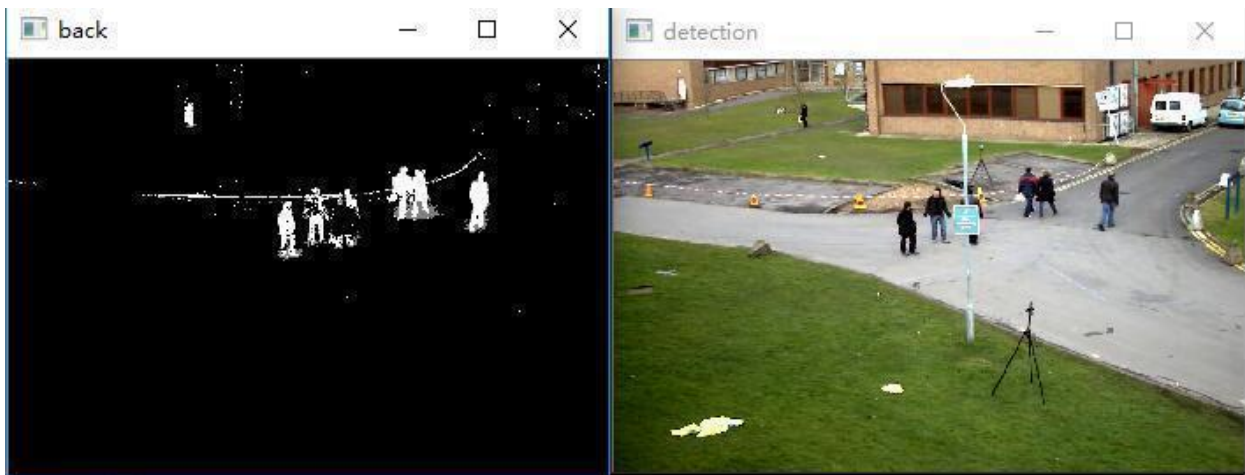
Fig. 2. An example of KNN algorithm operation on a digital video stream
