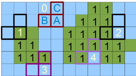
Figure 4. ABC mask and direction of sequential image (its green part) scanning
