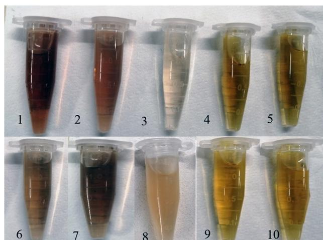
**Figure 1.** Synthesis of Ag and Fe nanoparticles exhibit color change. **First row** – solutions fabricated with leaf extracts (1 – NOL-Ag; 2 – NOL-Ag after 24 h; 3 – crude NOL extract; 4 – NOL-Fe; 5 – NOL-Fe after 24 h). **Second row** – solutions fabricated with flower extracts (6 – NOF-Ag; 7 NOF-Ag after 24 h; 8 – crude NOF extract; 9 – NOF-Fe; 10 – NOF-Fe after 24 h).
