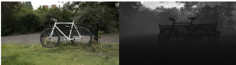
Fig. 3. Example of reconstruction of the bicycle, where densification procedure allows to represent thin spokes. Left figure is the color rendering mode, right is the depth rendering mode.
