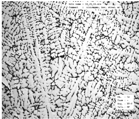
Fig. 1. AlCu4MgMn alloy microstructure before homogenization; enl: \times 100 .
