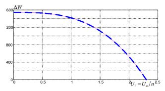
**Fig. 4.** Dependence of the difference between energies  $\Delta W$  accumulated in SC and LC, in the process of charge from the initial voltage  $U_f = U_n/n$  up to the final voltage  $U_f = U_n$ .
