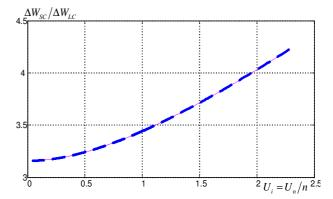
**Fig. 5.** Dependence of the ratio of energy doses accumulated in SC and LC during the charge from the voltage  $U_i = U_n/n$  to  $U_f = U_n$  on the value of initial voltage on the terminals of capacitors.
