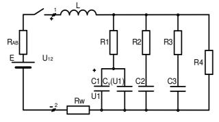
Fig. 1. Equivalent scheme of SC.
