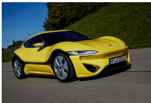
Fig. 3. RFB powered electric vehicle “QUANTINO 48VOLT”, developed by nanoFlowcell ( http://nanoflowcell.com/ ). This street legal prototype claims over 1,000 km range out of 85 kWh achieved by 2×95 L ionic liquid fuel.
