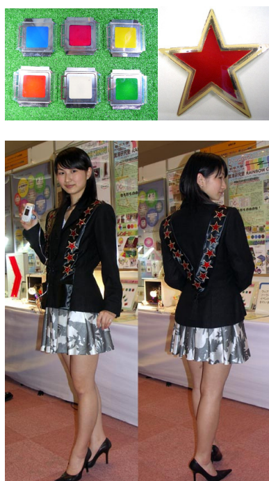
Fig. 1. Colorful plastic DSSCs and “wearable solar clothe” to power a mobile phone.
