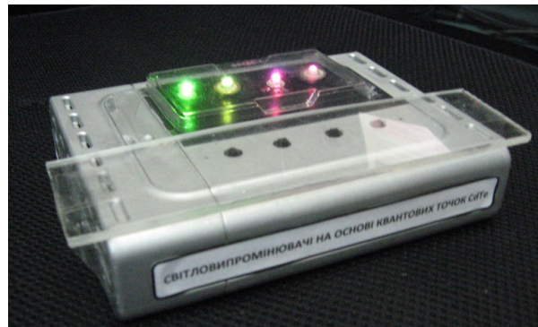
Fig. 3. Conversion semiconductor LED based on nc-CdTe.
