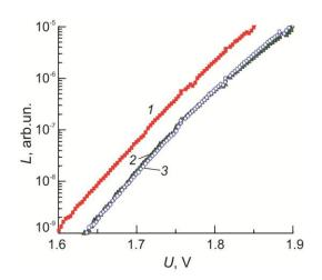
**Fig. 6.** Dependence of the luminosity on the applied voltage for the GaAs<sub>1-x</sub>P<sub>x</sub> diode (yellow): 1 - initial,  $2 - F = 3 \cdot 10^{14} \text{ cm}^{-2}$ ,  $3 - F = 5.9 \cdot 10^{14} \text{ cm}^{-2}$ .
