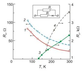
**Fig. 4.** Temperature dependences of the GaAs<sub>1-x</sub>P<sub>x</sub> orange parallel ( $R_p$ ) and series ( $R_s$ ) resistances for initial (I) and irradiated by 2 MeV electrons:  $2 - F = 2.64 \cdot 10^{16} \text{ cm}^{-2}$ ,  $3 - 2 \cdot 10^{14} \text{ cm}^{-2}$ ,  $4 - 9.5 \cdot 10^{15} \text{ cm}^{-2}$ .
