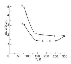
**Fig. 3.** Temperature dependence of the non-ideal coefficient *m* in irradiated orange  $\text{GaAs}_{1-x}\text{P}_x$  LED:  $l - F = 2 \cdot 10^{14} \text{ cm}^{-2}$ ,  $2 - F = 9.5 \cdot 10^{15} \text{ cm}^{-2}$ .
