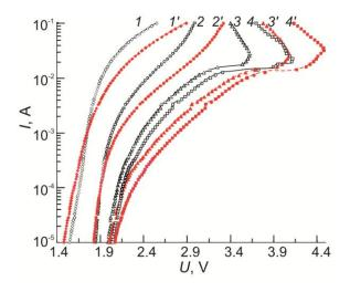
**Fig. 2.** Current-voltage characteristics of the orange GaAs<sub>1-x</sub>P<sub>x</sub> diode in the mode of the current generator at different sample temperatures: initial: I - 300 K, 2 - 180 K, 3 - 95 K, 4 - 77 K; irradiated (E = 2 MeV,  $F = 2.64 \cdot 10^{16}$  cm<sup>-2</sup>): I' - 300 K, 2' - 180 K, 3' - 95 K, 4' - 77 K.
