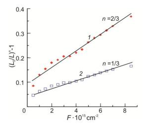
**Fig. 5.** Dependence of  $\left(\frac{L_0}{L}\right)^n - 1$  on fluence e-irradiation: *I* - yellow GaAs<sub>1-x</sub>P<sub>x</sub> diode, 2 - orange GaAs<sub>1-x</sub>P<sub>x</sub> diode.
