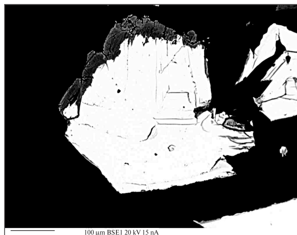
Fig. 5. White layered crystal of telluronevskite with secondary mineral related to montanite (?) (Poruba pod Vihorlatom)
