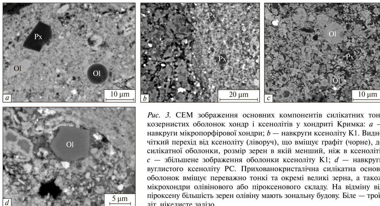
Fig. 3. SEM image of main components of the silicate fine-grained chondrule and xenoliths rims within the Krymka chondrite: a — around microporphyritic chondrule; b — around the xenolith K1. Clear transition from the graphite-bearing (black) xenolith (left) toward the silicate rim is visible. Grain size of the silicate rim is smaller than that of the xenolith; c — enlarged image of the xenolith K1 rim; d — around the carbonaceous xenolith PC. A cryptocrystalline silicate groundmass of the rims includes mostly fine grains, minor coarse grains and olivine and pyroxene microchondrules. Unlike pyroxene grains most olivine ones are zones. White — troilite, Fe, Ni-metal
