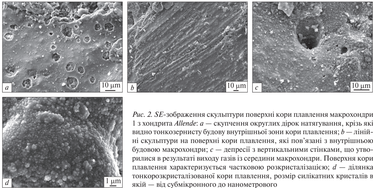
Fig. 2. SE-images of melted crust surface sculptures of the macrochondrule 1 from the Allende chondrite: a — an accumulation of the round tension holes with visible a fine-grained structure of the melted crust inner zone; b — linear sculptures on the melted crust surface, related to a macrochondrule internal texture; c — depressions with vertical walls, formed in result of gas outlet from the macrochondrule internal zone. The melted crust surface is characterized by a partial recrystallization; d — an area of the fine-recrystallized melted crust, with silicate crystals ranging in a size from submicrons to nanometers
