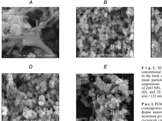
**F i g. 1.** SEM images of dry powders of conventional ZnO, cZnO (A) and ZnO in the form of nanoparticles, ZnO NPs (B, mean particle size <70 nm) and those of suspensions with different concentrations of ZnO NPs, 5 mg/5 cm³ (C), 10 mg/5 cm³ (D), and 20 mg/5 cm³ (E); mean particle size >133 nm.
