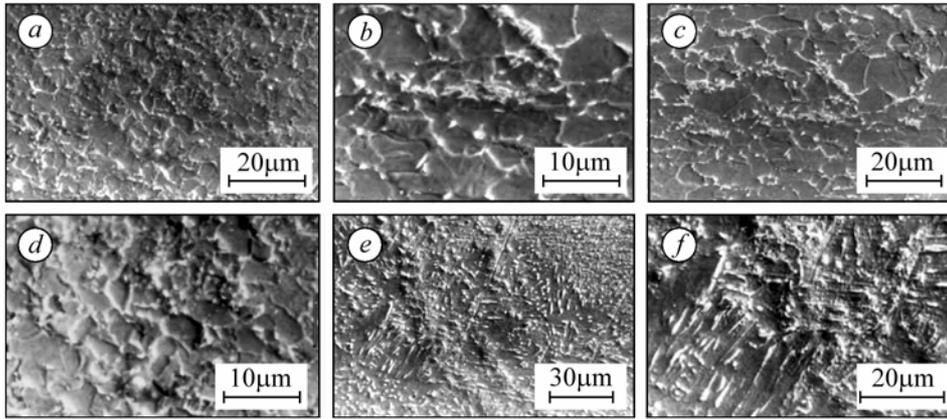
Fig. 3. SEM microphotographs of different zones of microstructure of welded steel Nb/Ti-A: *a* – base metal (ferrite + pearlite); *b* – magnification of photograph *a*; *c* – zone of normalization; *d* – magnification of photograph *c*; *e* – WM zone; *f* – magnification of photograph *e*.
