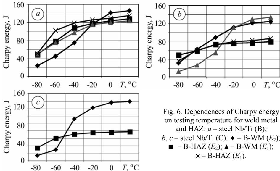
Fig. 6. Dependences of Charpy energy on testing temperature for weld metal and HAZ: a – steel Nb/Ti (B); b, c – steel Nb/Ti (C):  $\blacklozenge$  – B-WM ( $E_2$ );  $\blacksquare$  – B-HAZ ( $E_2$ );  $\blacktriangle$  – B-WM ( $E_1$ );  $\times$  – B-HAZ ( $E_1$ ).
