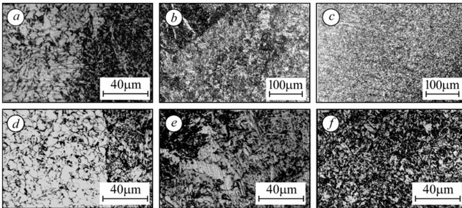
Fig. 4. HAZ microstructure of welded steel Nb/Ti-B: *a-c* –  $E_1 = 7.5$  kJ/cm; *d-f* –  $E_2 = 21$  kJ/cm.
