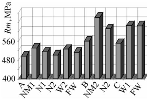
Fig. 5. Compared values of tensile strength of base metal and welded joints made by: E-process with electrode quality NM1, NM2, N1, N2; MAG-process with electrode wire W1, W2, FW. Designations: A, B, C – steel type Nb/Ti (X65); NM1, NM2, N1, N2 – coated electrode; W1, W2 – classical electrode wire; FW – filled wire.
