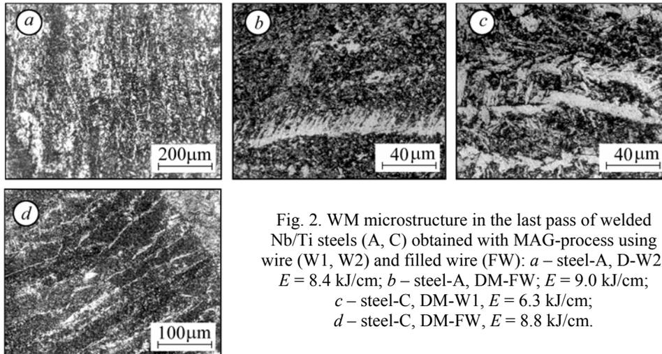
Fig. 2. WM microstructure in the last pass of welded Nb/Ti steels (A, C) obtained with MAG-process using wire (W1, W2) and filled wire (FW): a – steel-A, D-W2;  $E = 8.4$  kJ/cm; b – steel-A, DM-FW;  $E = 9.0$  kJ/cm; c – steel-C, DM-W1,  $E = 6.3$  kJ/cm; d – steel-C, DM-FW,  $E = 8.8$  kJ/cm.
