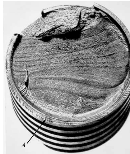
Fig. 1. Failure emanating from a column with a square thread of a friction screw press (diameter of the column is 97.5 mm; outer and internal diameter of the square thread equals 96 mm and 88.1 mm, respectively).
