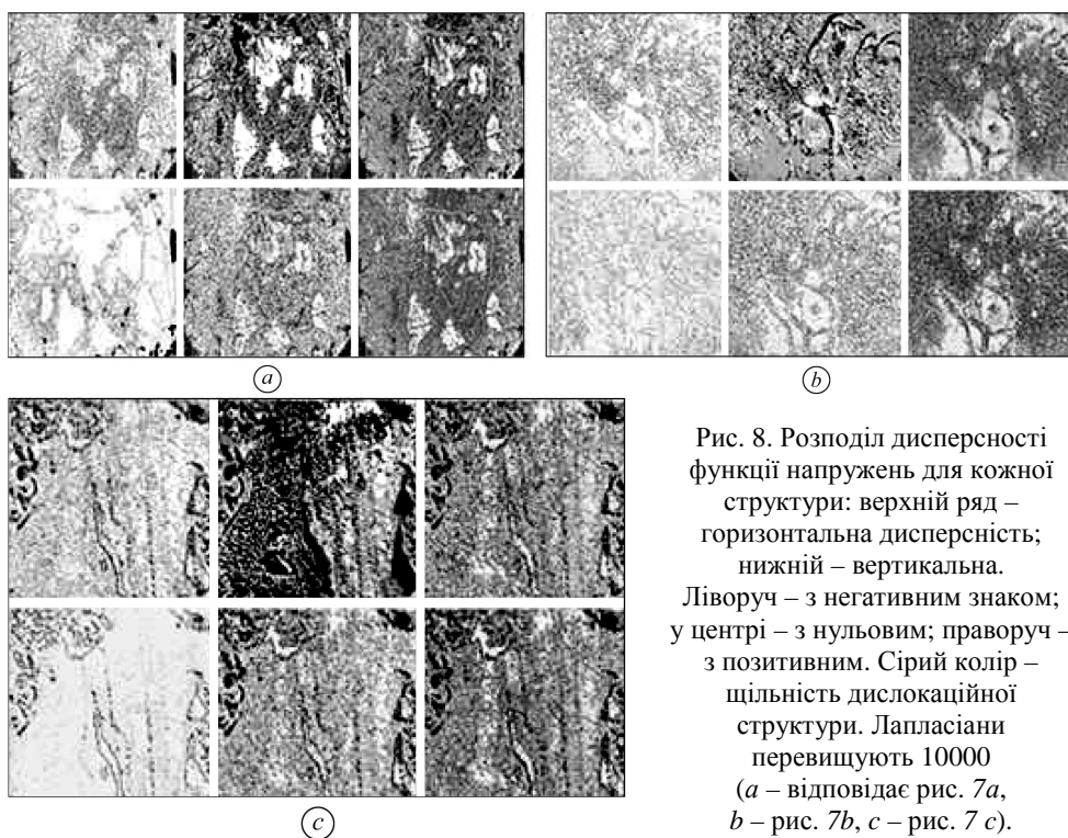
Fig. 8. Distribution of stress functions for each structure: top row shows horizontal dispersity; bottom row – vertical dispersity. The left-hand part indicates negative dispersity; the central part – zero dispersity; the right-hand part – positive. Dislocation structure density is given in grey. The value of Laplacian operators exceeds 10000 ( a – corresponds to Fig. 7 a , b – Fig. 7 b , c – Fig. 7 c ).
