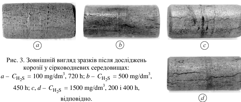
Fig. 3. External view of samples after corrosion tests in hydrogen sulfide media: a – C_{H_2S} = 100 mg/dm^3 , 720 h; b – C_{H_2S} = 500 mg/dm^3 , 450 h; c, d – C_{H_2S} = 1500 mg/dm^3 , 200 і 400 h, respectively.
