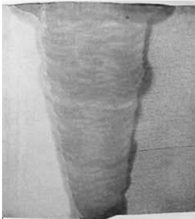
Fig. 4. Welded joint macrorecording.
