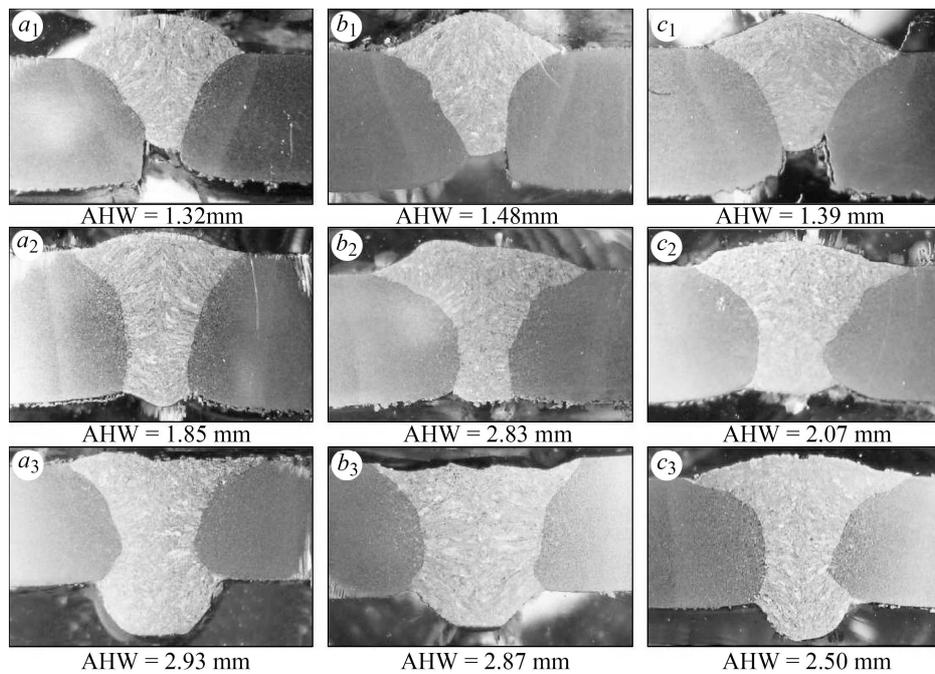
Fig. 1. The measured value for AHW in experiments.
