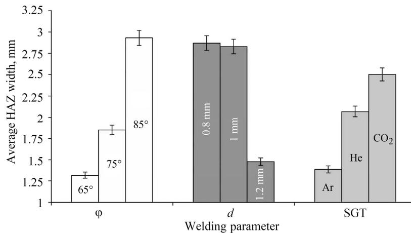
Fig. 2. The effect of welding parameters on AHW.
