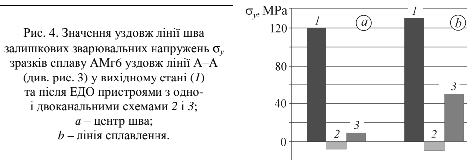
Fig. 4. The value of residual welding stresses \sigma_y of AMg6 alloy samples along the line A–A (see Fig. 3) in the initial state (1) and after EDT by single- and two-channel schemes 2 and 3; a – the center of the weld; b – fusion line.
