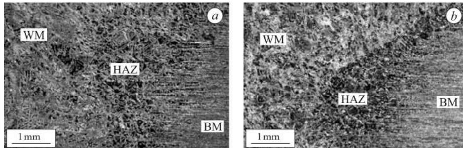
Fig. 2. Micrography of the 2205 DSS welds made without magnetic field (0 mT) (a) and under the effect of a magnetic field of 3 mT (b) [15].
