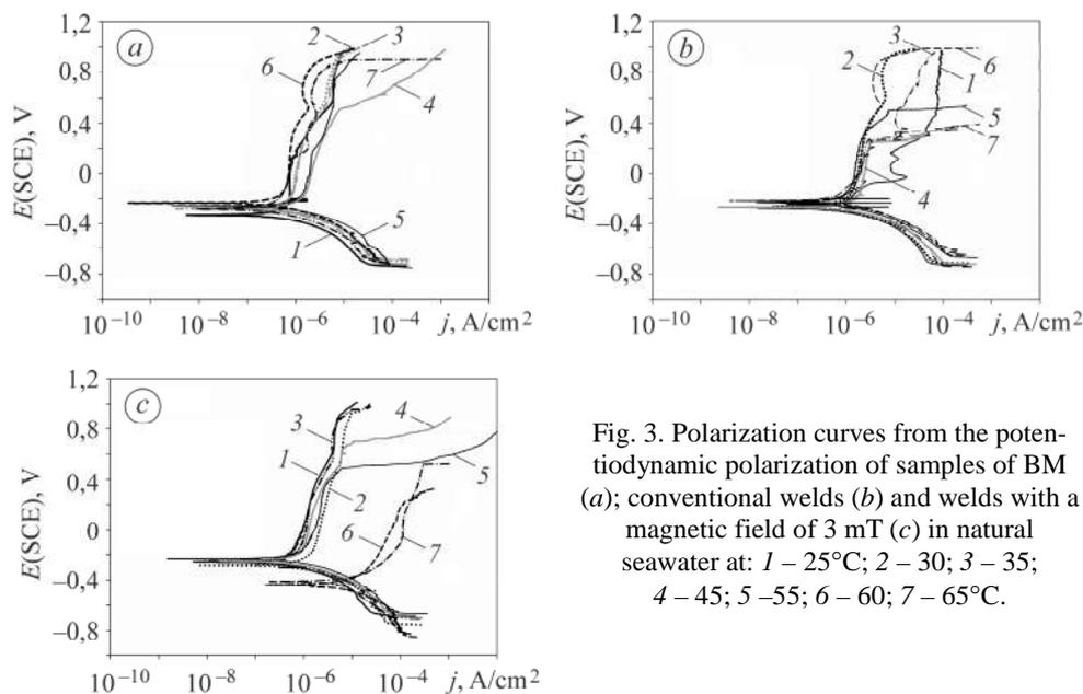
Fig. 3. Polarization curves from the potentiodynamic polarization of samples of BM (a); conventional welds (b) and welds with a magnetic field of 3 mT (c) in natural seawater at: 1 – 25°C; 2 – 30; 3 – 35; 4 – 45; 5 – 55; 6 – 60; 7 – 65°C.
