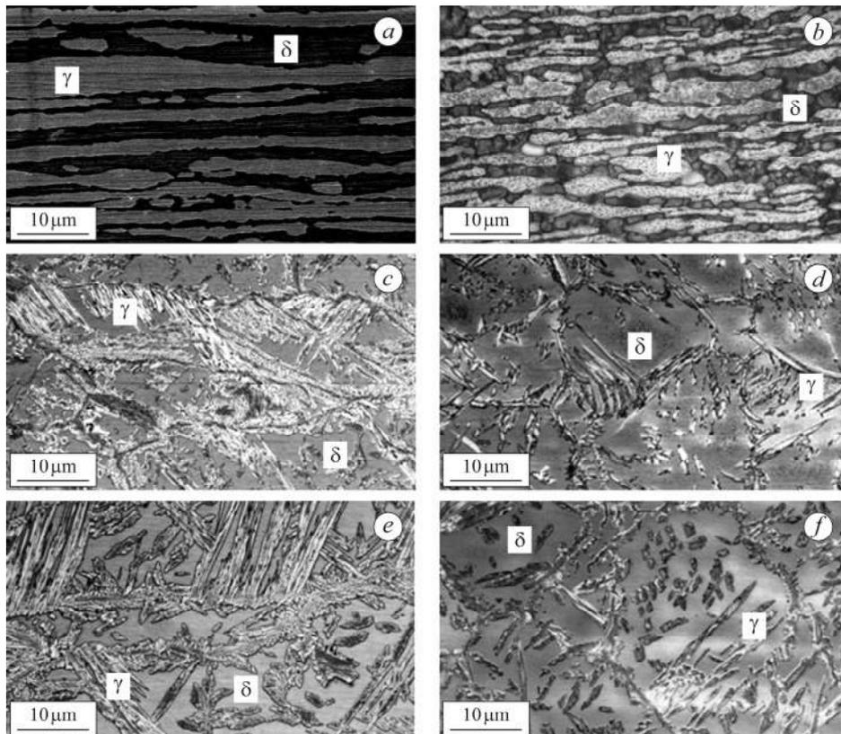
Fig. 1. Microstructure ( $\times 2000$ ) of the BM and welded joints *a* – BM surface area; *b* – BM transverse area; FZ (*c*) and HAZ (*d*) of the welded joints with the application of a magnetic field of 3 mT; FZ (*e*) and HAZ (*f*) of welds made without the application of a magnetic field.
