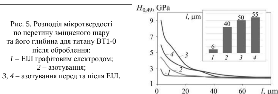
Fig. 5. Cross-section distribution of microhardness and depth of hardened layer for BT1-0 titanium after treatment: 1 – ESA with a graphite electrode; 2 – nitriding; 3, 4 – nitriding before and after ESA.
