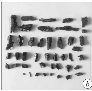
Fig. 4. Fragmentation of cylinders manufactured of 60C2A steel after their static explosion tests: a – quenching at 820°C and cooling in water; b – preliminary hydrogen-charging to C_H = 4.36 ppm.
