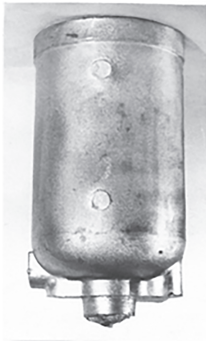
Figure 3. Casting of filter housing part obtained by LowPressure die casting
