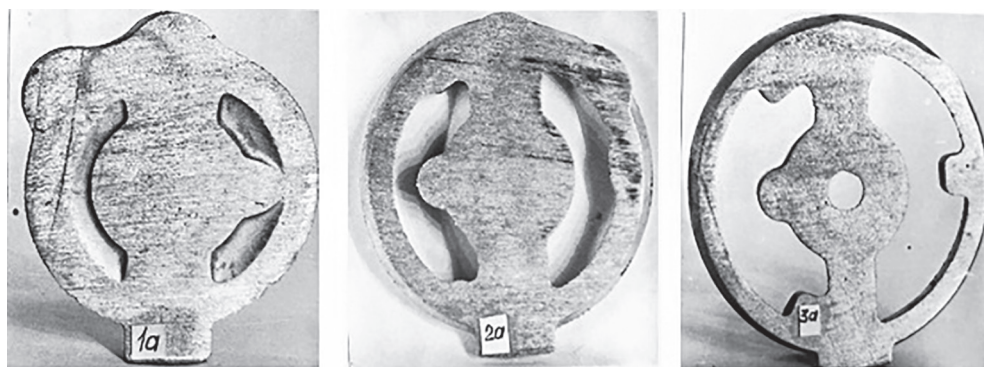
Figure 5. Casting sections produced with central metal feeding: 1 a – 30 mm from lower end of the casting; 2 a – 45 mm from lower end of the casting; 3 a – 60 mm from lower end of the casting
