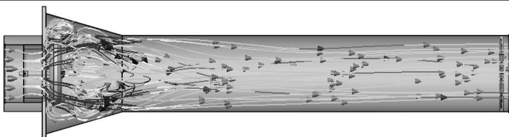
Fig. 4. Velocity fields through the anemostat, funnel and part of the cylinder for a 5 mm gap
