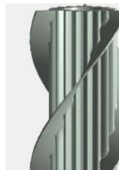
Fig. 13. Fuel elements with longitudinal finning and helical plates
