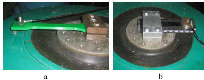
Fig. 3. Photos of the samples fixed on the shaker: a – sample from PLA; b – a three-layer plate
