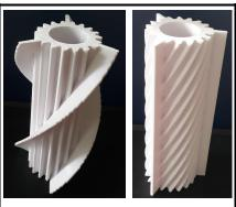
Fig. 5. Fuel elements models made on a 3D printer
