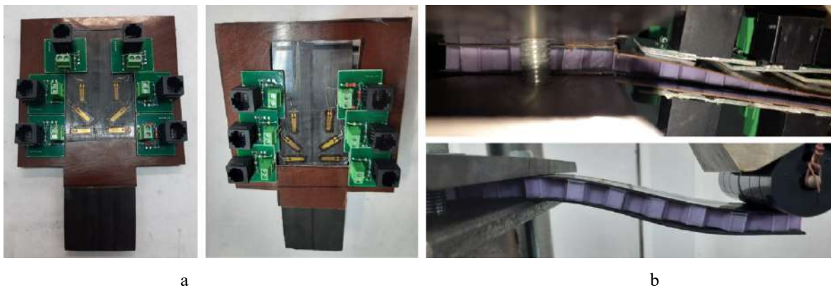
Fig. 6. A sample of a three-layer honeycomb panel before and after loading: a – photo of housings with installed strain gauges and microcircuits; b – typical destruction of the sample
