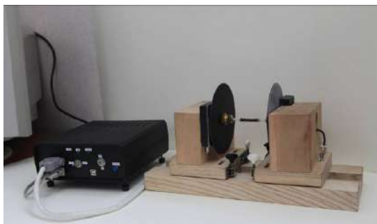
Fig. 4. The stand of the two-mass electromechanical tracking system
