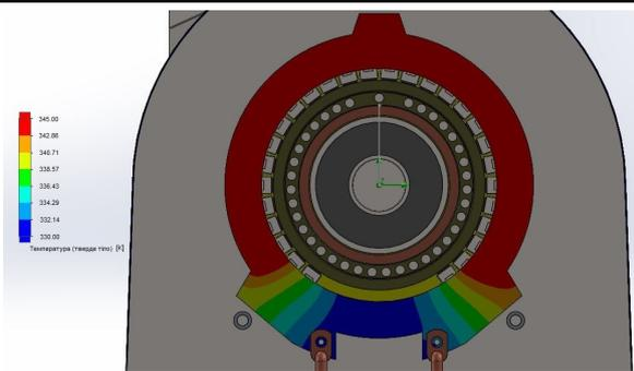
**Fig. 9. Bus No. 1 temperature**
