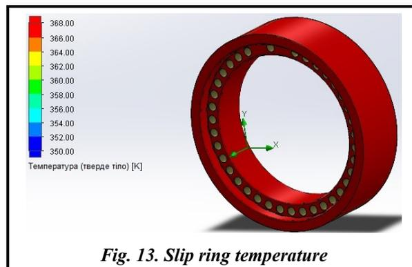
Fig. 13. Slip ring temperature
