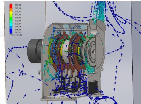
**Fig. 8. Flow trajectories and temperatures**
