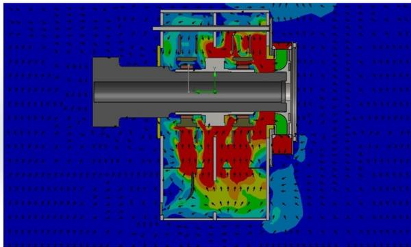
**Fig. 7. Cross section and flow velocity**
