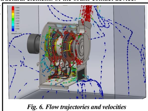
Fig. 6. Flow trajectories and velocities
