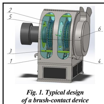
*Fig. 1. Typical design of a brush-contact device*
