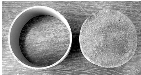
Fig. 1. A typical rock-like disk specimen.
