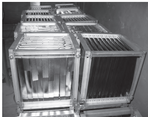
Fig. 7. Elements - blocks of ribbon packings for industrial contact heat recovery apparatus
