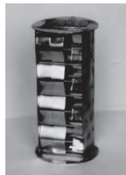
Fig. 3. Laboratory sample of amorphous metal ribbon packing (side wall is removed)
