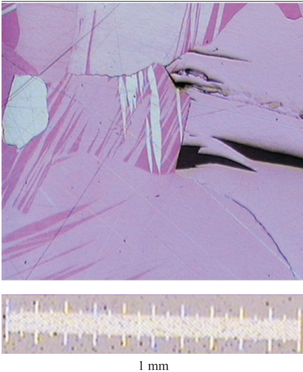
Fig. 6. (Color online) False color optical image of Bi polycrystalline sample studied in Ref. 4 and the present work.
