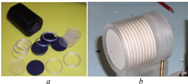
Fig. 40. The axially symmetrical microwave 1D photonic crystals: for ambient space research: ferrite/polystyrene/air-gap MPC (a); teflon/quartz PC; diameter of disks is about \approx 5-7 \lambda (b).
