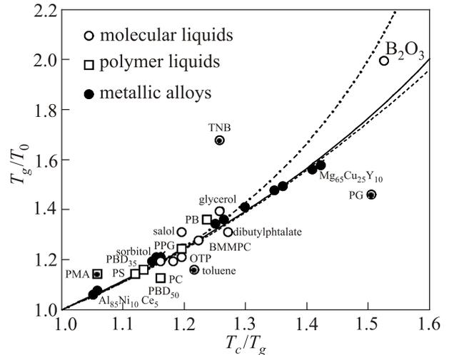
Fig. 4. Universal equations for the glass-transformation characteristic temperatures. Symbols are described in Fig. 3. The solid line is given by Eq. (17) with the material-independent parameter  $m_g^*/m_c^* = 2.17$ . The dashed and dashed-dotted lines are drawn through Eqs. (18) and (19), respectively.
