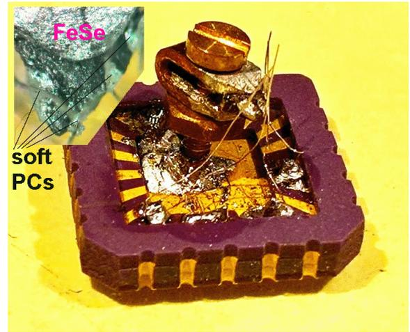
*Fig. 1.* (Color online) FeSe sample clamped within the copper clip by means of the brass screw and the nut. To create good thermal contact the screw itself was soldered to the base plate of the 20-lead chip and coupled electrically with two such leads. Inset (left top corner): Enlarged image of the FeSe sample with four “soft” contacts attached.
