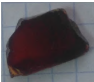
Fig. 1. Typical photo image of studied \text{Tl}_4\text{HgI}_6 crystal (as-grown).
