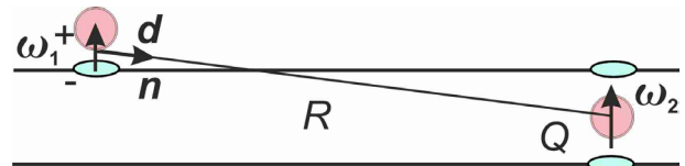
Fig. 5. Interaction of the adatom's dipole and quadrupole formed by the intercalating atom in semiconducting bigraphene according to (9).
