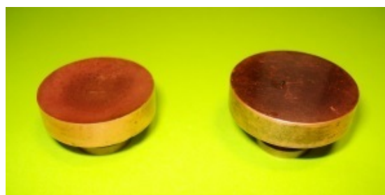
Fig. 3. Set of mirrors with the different radius of curvature for two-mirror open cavity in the radiospectrometer BURAN.
