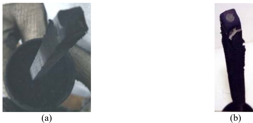
Fig. 2. General view of the consumable anode electrode after its partial evaporation: a) SIGE graphite brand; b) FGDG-7 graphite brand
