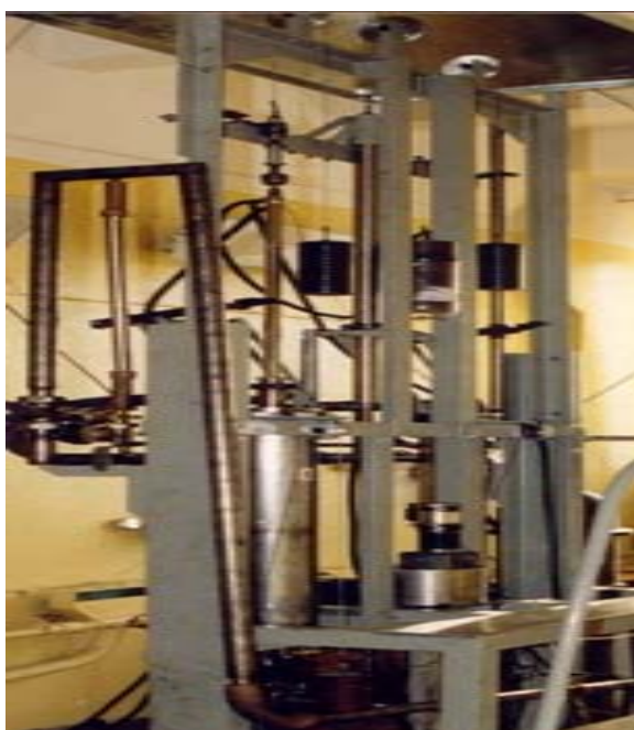
Fig. 1. Photo of the equipment for plasma-chemical synthesis of CNS in a gaseous environment
