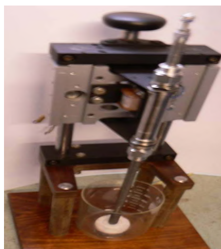
Fig. 3. Photo of the equipment for plasma-chemical synthesis of CNS in a liquid environment
