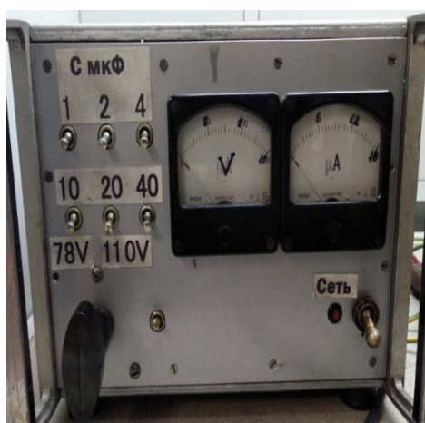
Fig. 3. Photo of the equipment for plasma-chemical synthesis of CNS in a liquid environment
