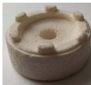
Fig. 20. 3D product from a mechanical mixture (ceramic–CNS) using CJP technology
