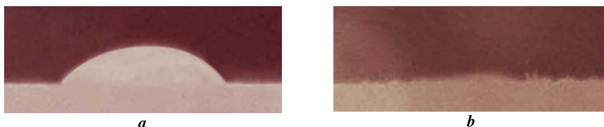
Fig. 1. Wetting of ZnO-ceramics with Ge melt with various holding times at 1000°C: a – 0; b – 5 min
