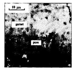
Fig. 3. CEM-picture of sample of the garnet ceramic (sample 1H, Table 1).
