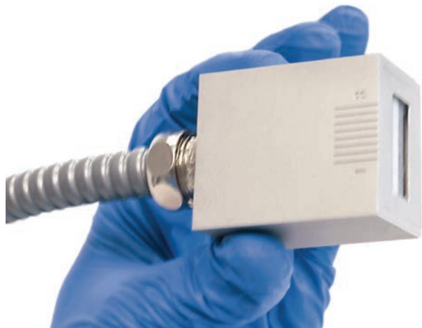
Figure 6. Eight-channel array detector head. If combined with an excitation laser with a line-shaped beam profile, it increases the scanning speed by a factor of 8.
