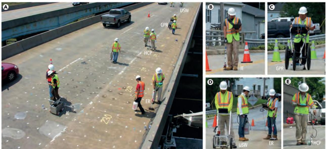
Figure 1. Manual NDE data collection on a bridge deck (a) using the following NDE technologies: (b) impact echo; (IE); (c) ground penetrating radar (GPR); (d) ultrasonic surface waves (USW) and electrical resistivity (ER); (e) half-cell potential (HCP)
