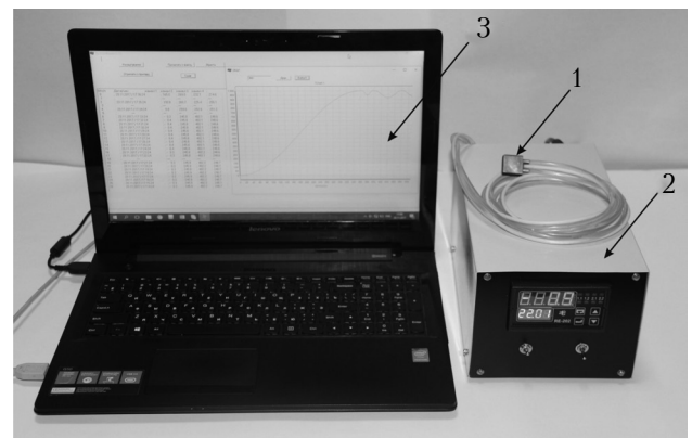
Fig. 1. Thermoelectric device with electronic control unit for the diagnostics of inflammatory processes in the human body:
