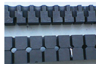
Fig. 7. Photograph of the upper and lower parts of the graphite cassette used to form “ n -Si — Al+Si melt — p^+ -Si” structures
