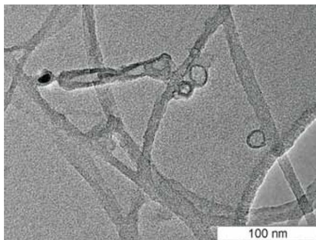
Fig. 7. TEM-image of the non-covalent hybrid of 5'-pyrene conjugate (IIa) with SWNT-HMDA-FITC
