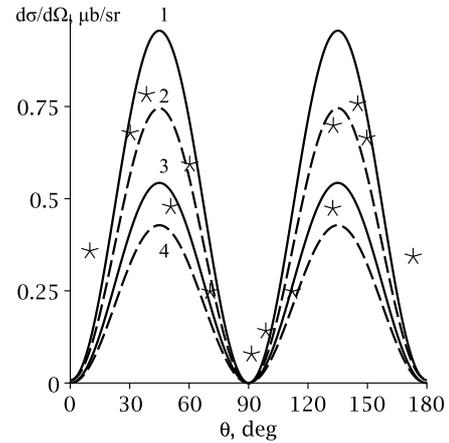
**Fig. 4.**  ${}^4\text{He}(\gamma, d)d$  differential cross section at  $E_\gamma = 40$  MeV, solid lines take the contact part into account, dash lines don't take the contact part into account, curves 1, 2 were calculated, by using the Argonne parametrization, curves 3, 4 were calculated, by using the Urbana parametrization, and \* - experimental data [24]
