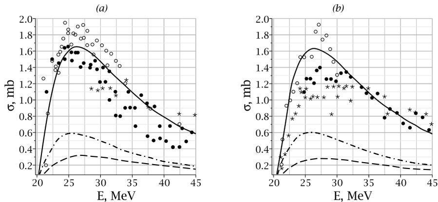
**Fig. 8.** Dependence of the total cross sections  $\sigma$  for the reactions  ${}^4\text{He}(\gamma, p)\text{T}$  (a) and  ${}^4\text{He}(\gamma, n){}^3\text{He}$  (b) on the photon energy in the interval from 20 to 44 MeV. Experimental data are from [26]
